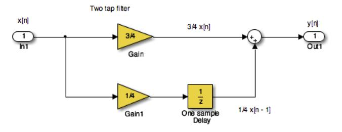
This system is available as a Simulink model discrete\_system.slx
