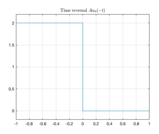
The sign on the function argument -t causes the whole signal to be reversed in time. Note that another way of looking at this is that the signal is mirrored about the  $\boldsymbol{y}$  axis.
