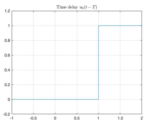
This is a *time delay* ... note for  $u_0(t-T)$  the step change occurs T seconds **later** than it does for  $u_o(t)$ .
