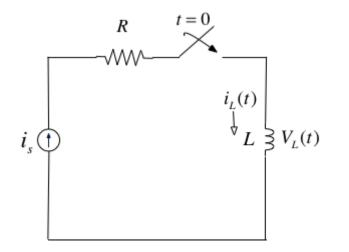
In the circuit shown above, the switch is closed at time t = 0 and  $i_L(t) = 0$  for t < 0. Express the inductor current  $i_L(t)$  in terms of the unit step function and hence derive an expression for  $v_L(t)$ .
