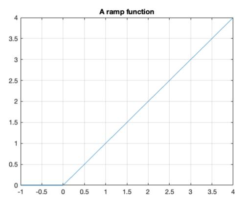
This type of signal is called a ramp function. Note that it is the integral of the step function (the resistor-capacitor circuit implements a simple integrator circuit).
