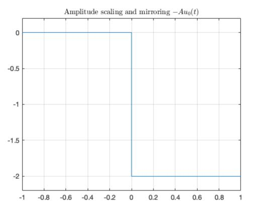
Note that, because of the sign, the signal is mirrored about the x axis as well as being scaled by 2.
