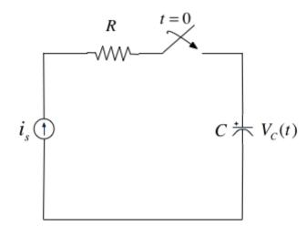
In the circuit shown above  $i_s$  is a constant current source and the switch is closed at time t = 0.
