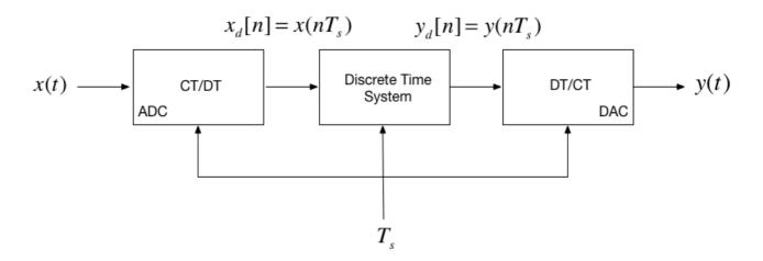
In the remainder of this course we turn our attention to how we model and analyse the behaviour of the central block in this picture.
