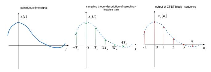
The signals we process in discrete time systems are sequences of values x[n] where n is an index.
