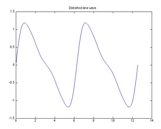
This can occur in the line voltages of an industrial plant that makes heavy use of nonlineear loads such as electric arc furnaces, solid state relays, motor drives, etc (E.g. Tata Steel!)
