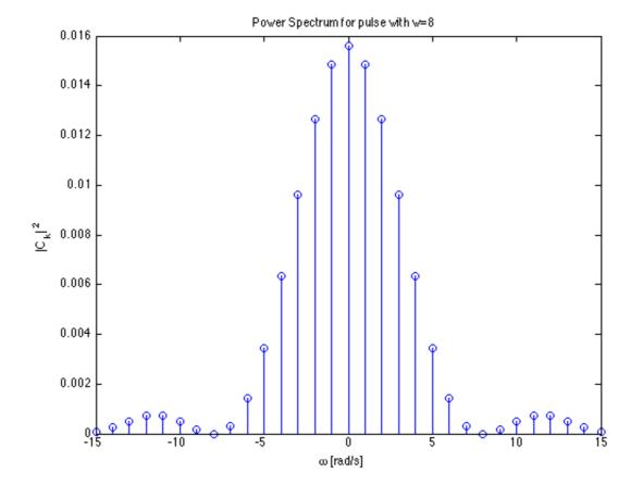
This is the power spectrum for a pulse with width T/8.
