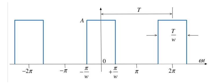
What happens when the pulses to the left and right of the centre pulse become less and less frequent? That is what happens when  $T \to \infty$ ?
