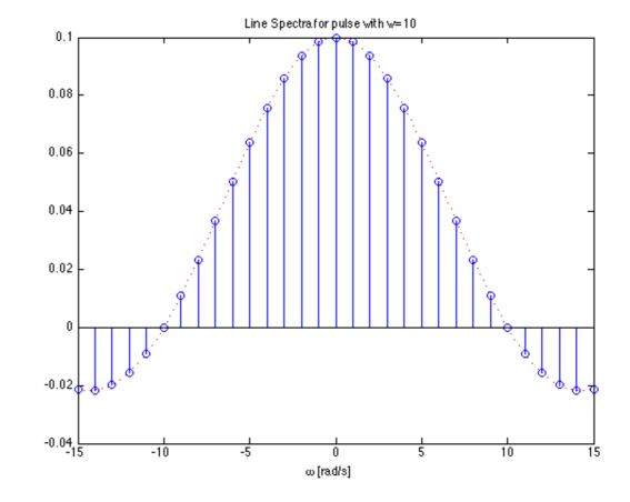
$\Omega_0 = 1 \text{ rad/s}; w = 10; T = 2\pi \text{ s}; T/w = \pi/5 \text{ s}.$
