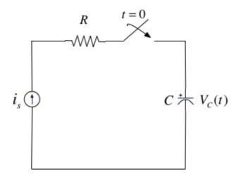
In the circuit shown above  $i_s$  is a constant current source and the switch is closed at time t = 0.
