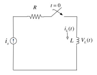
In the circuit shown above, the switch is closed at time t = 0 and  $i_L(t) = 0$  for t < 0. Express the inductor current  $i_L(t)$  in terms of the unit step function and hence derive an expression for  $v_L(t)$ .
