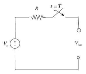
Express the output voltage  $v_{out}$  as a function of the unit step function, and sketch the appropriate waveform.
