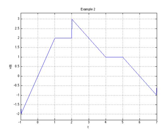
(1) Express the voltage waveform v(t) shown above as a sum of unit step functions for the time interval -1 < t < 7 s
